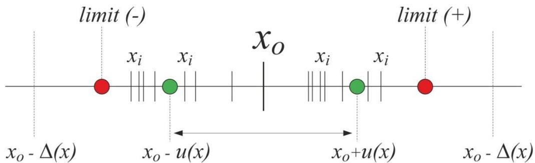
Fig. 26. Weighing limits using measurement uncertainty
