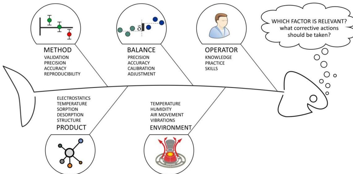
Fig. 43. Ishikawa diagram - sources of errors in mass measurements.
