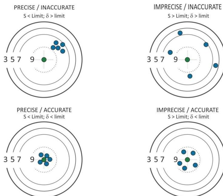
Fig. 6. Accuracy and precision measurement
