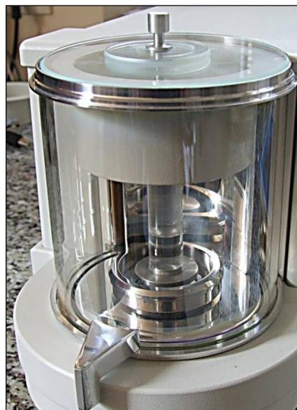
Fig. 42. Weighing liquid by means of so called evaporation ring, designed to check piston pipettes using balance
