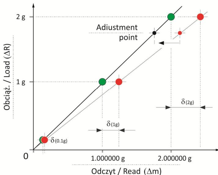
Fig. 34. Adjustment as sensitivity correction of the microbalance
