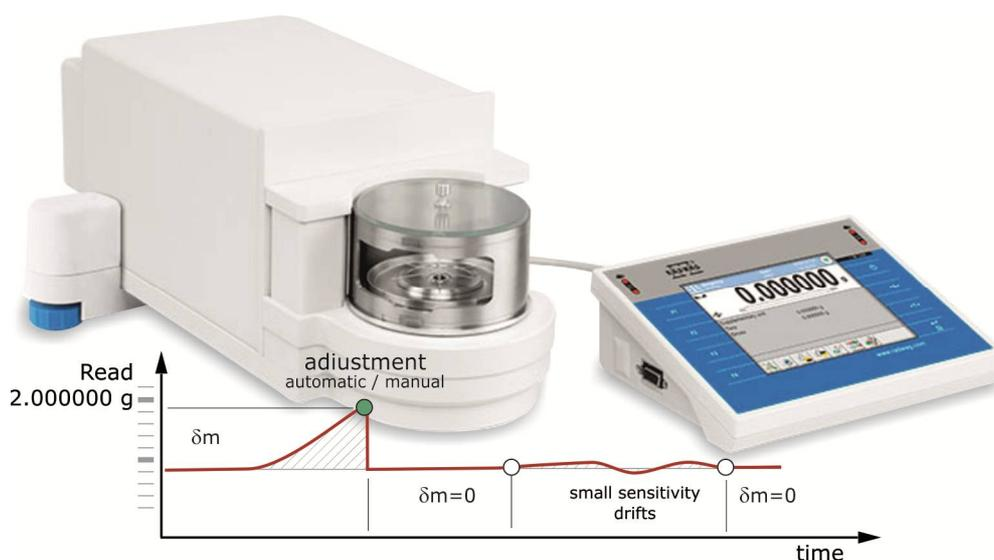
Fig. 33. Principle of balance adjustment operation
