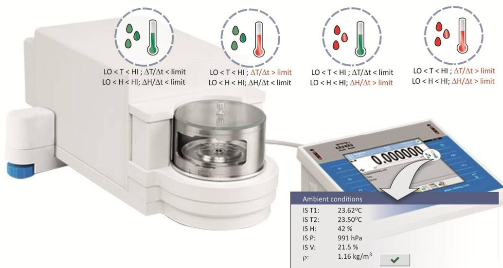
Fig. 13. Environmental conditions module for ultra-microbalances and microbalances
