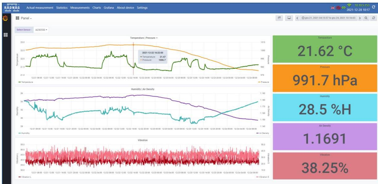
Fig. 12. Detailed analysis of environmental data for the selected period
