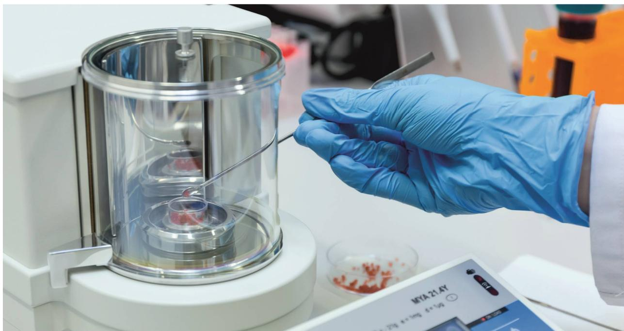
Fig. 10. Mikrcobalance – powder weighing
