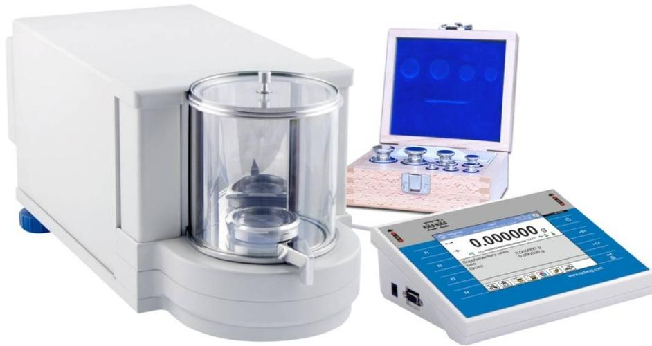
Fig. 44. Microbalance and standard mass
