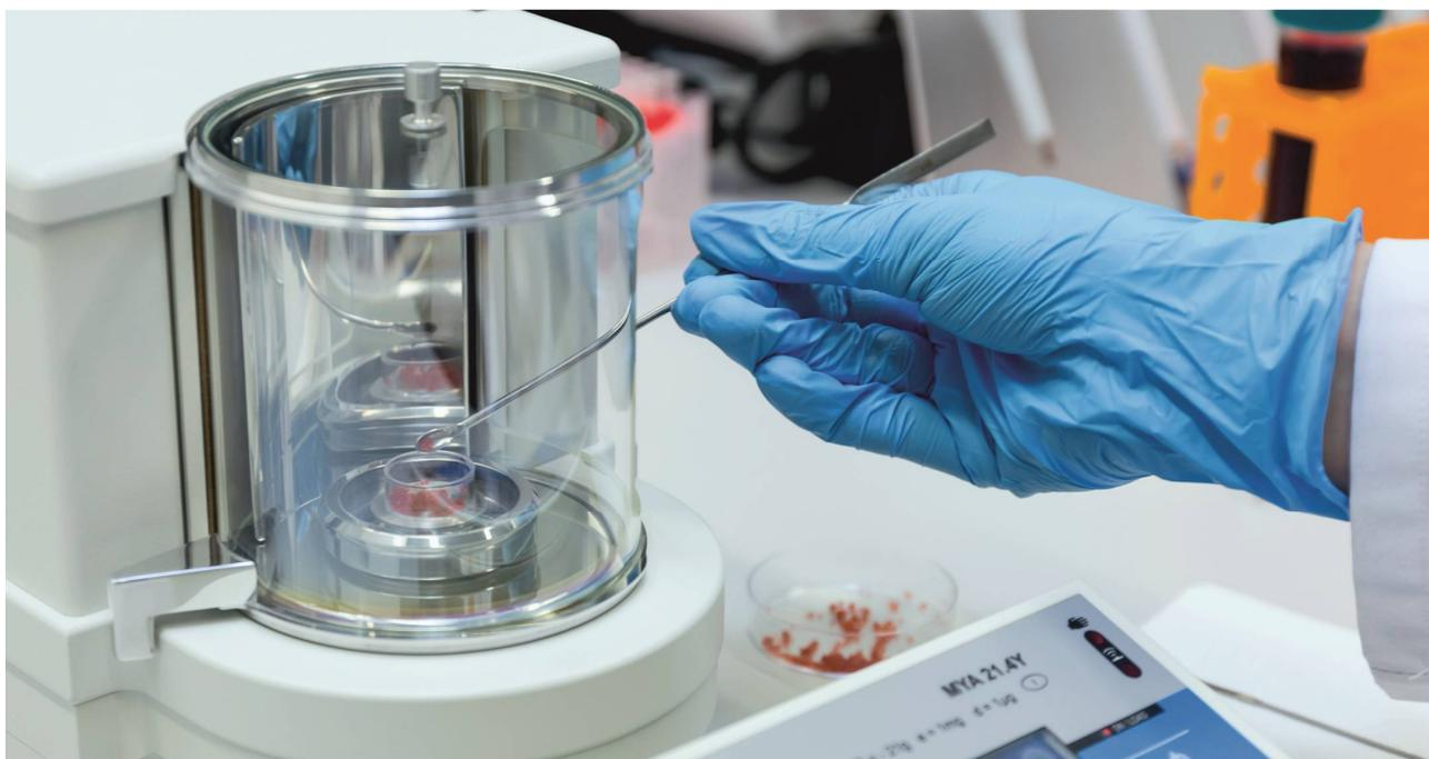
Fig. 10. Mikrcobalance – powder weighing
