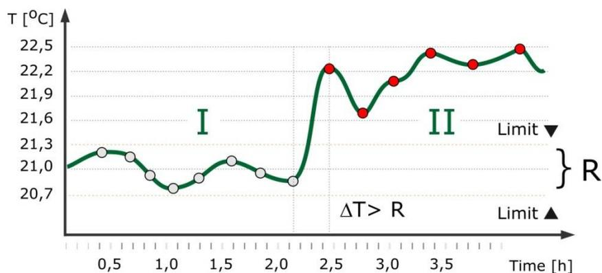
Fig. 5. Temperature variation dynamics (I- stability period, II – dynamic changes period)
