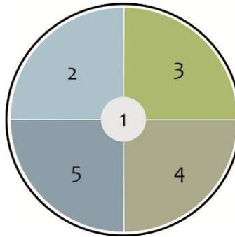
Fig. 28. Weighing pan – eccentricity testing points (acc. to EN 45501 test shall be performed for points 2-5, acc. to EURAMET for points 1-5)
