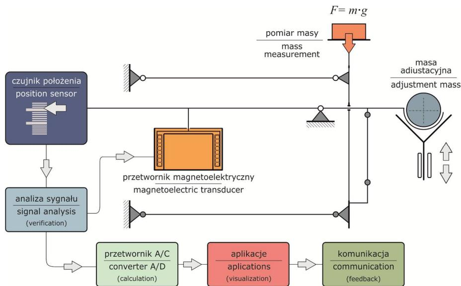
Fig. 22. Scheme of the balance of the magnetolectric processing system
