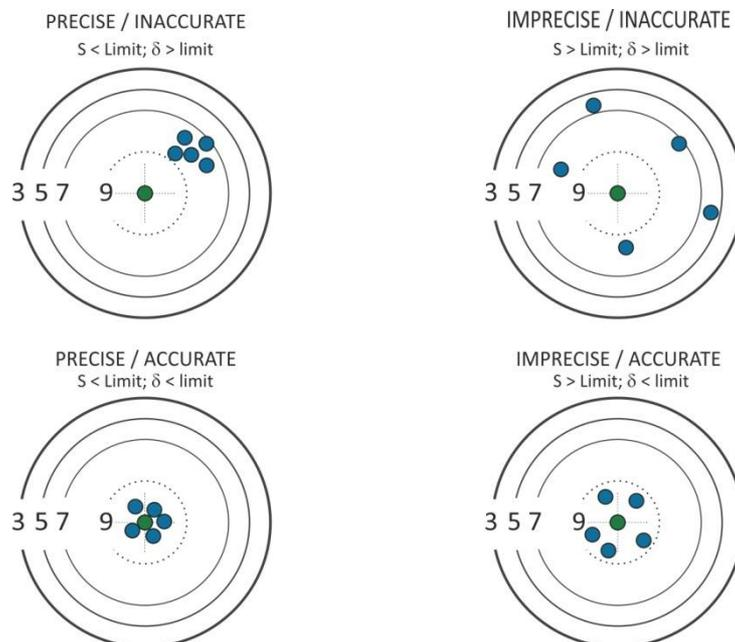
Fig. 6. Accuracy and precision measurement
