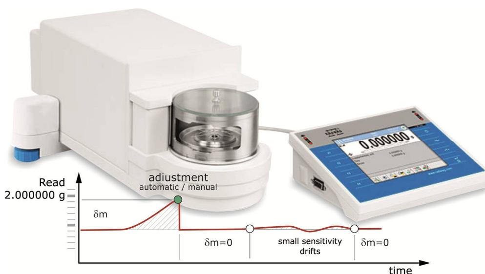
Fig. 33. Principle of balance adjustment operation
