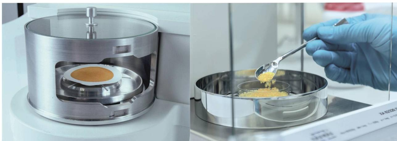
Fig. 18. Microbalance MYA 2.4Y.F.A PLUS – filter mass measurement, XA 82/220.4Y – powder weighing
