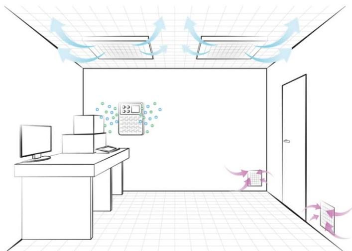
Fig. 16. An example of dispersed air conditioning.
