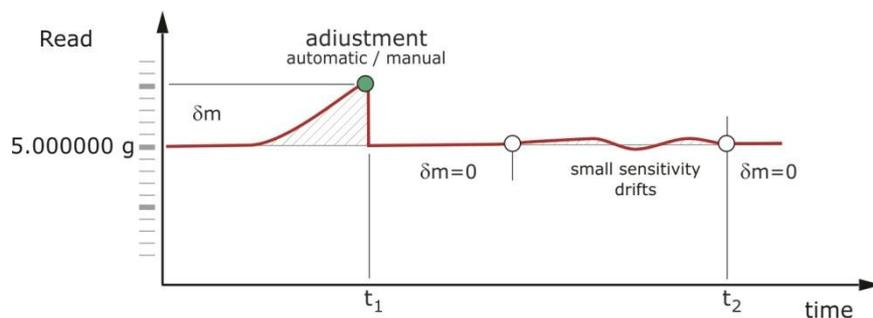
Fig. 17. Correction of accuracy of indications by means of automatic adjustment
