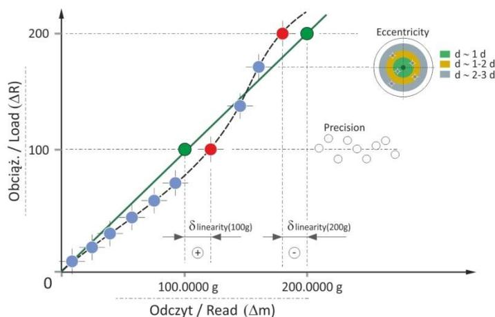
Fig. 32. Example of balance linearity
