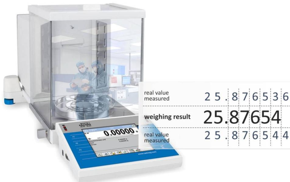
Fig. 7. Rounding of the measurement result of devices with digital indication
