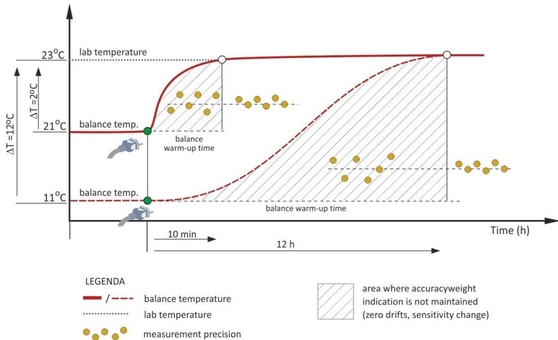
Fig. 4. Balance parameters change over acclimatization period
