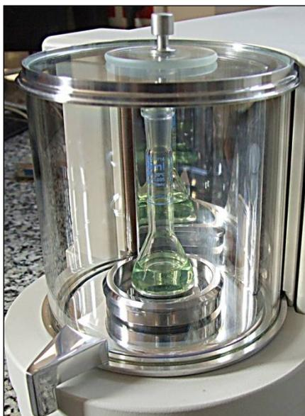
Fig. 41. Weighing liquid by means of vessel with a tapered inlet, liquid evaporation in course of weighing limited
