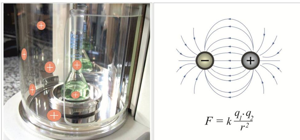
Fig. 20. Unbalanced electrostatic charges, Coulomb law
