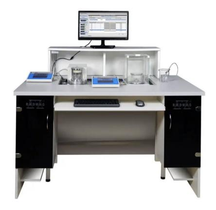
Photo 11. Piston pipette check and calibration stand.
