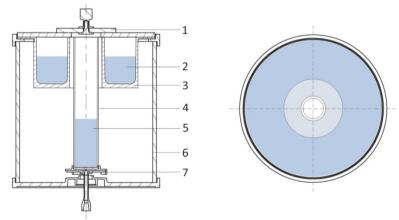
Photo 10. Steam curtain sketch for MYA microbalances and XA analytical balances
