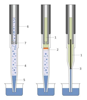
Photo 15. Liquid collection for various pipettes
