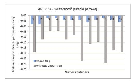
Photo 24. Liquid evaporation from the weighing vessel in the AP 12.5Y system
