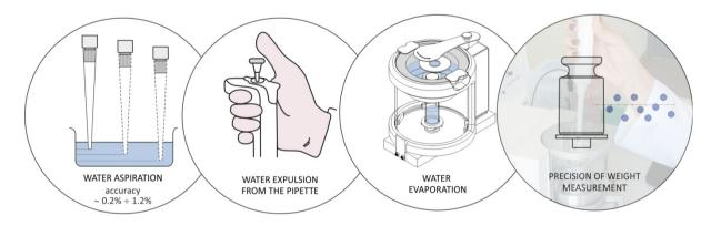
Photo 14. Sources of errors while pipetting
