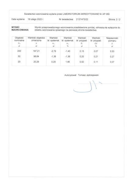
Photo 26. Single-channel pipette calibration certificate - results
