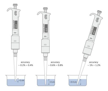
Photo 17. Potential measurement mistakes while collecting water
