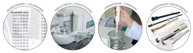
Photo 5. Piston pipette life cycle
