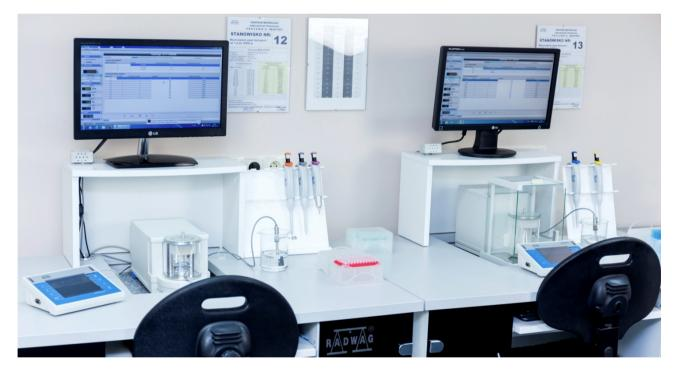
Photo 16. Various-volume piston pipette checking stand
