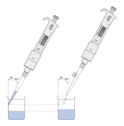
Photo 18. Method of expelling liquid from pipette
