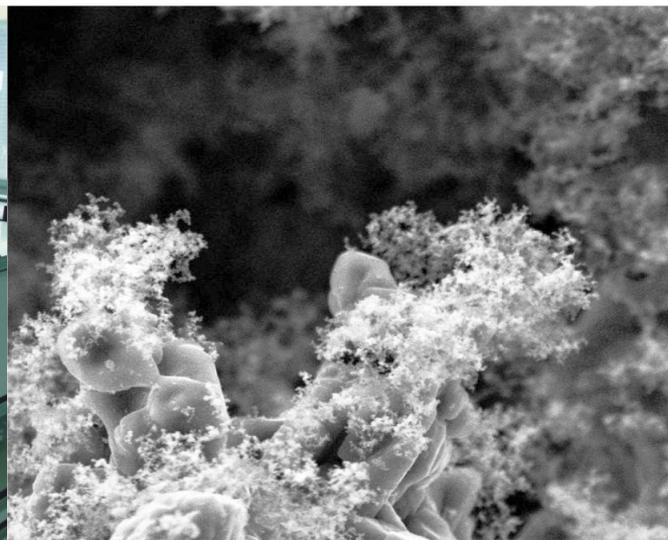
Scanning electron micrograph of diesel engine particulate matter captured in the pore of a ceramic wall-flow filter.
