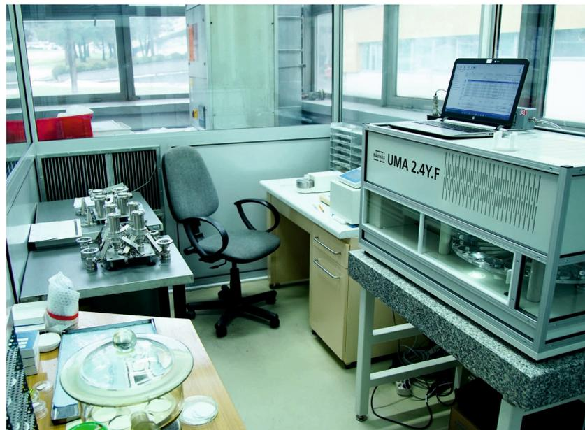
Weighing room – automatic and manual weighing system
