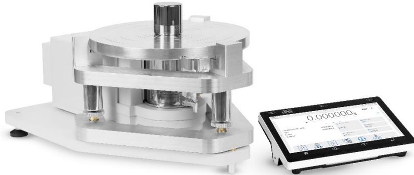
The **susceptometer** by **RADWAG** is used to measure magnetic susceptibility and magnetisation of E1-class weights or lower-class weights as per OIML R111. In view of its modular structure, once the suitable module has been disassembled, **the susceptometer** can be used as a mass comparator or balance/scale.
