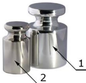
Set of mass standards for determining density of air (1) – aluminum standard, (2) – stainless steel standard
