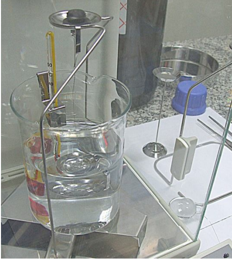
Solid body density determination (weighing in the air)
