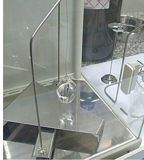
Liquid density determination (weighing the plunger in the air)
