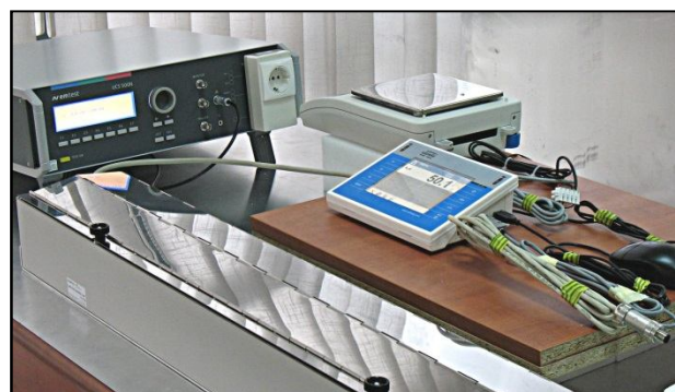
Testing the balance resistance to interference
