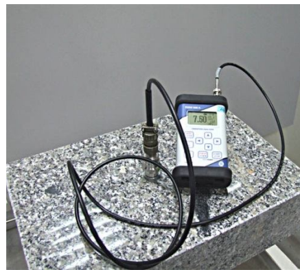
Testing vibrations of a granite slab
