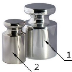
Mass standards kit for air density determination (1)- aluminium standard, (2) - steel standard
