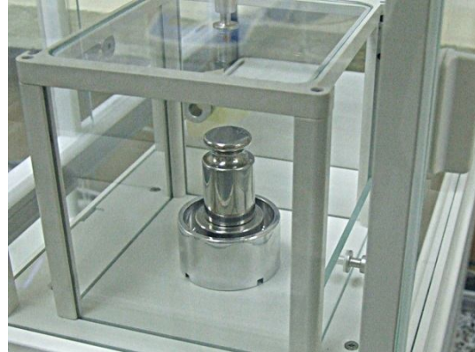
the weighing pan shield in the mass comparator
