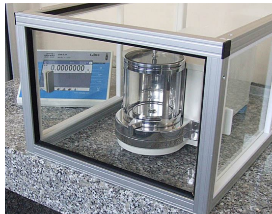
Grid weighing pan, external shield of the microbalance
