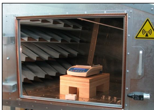
Testing the balance resistance in GTEM chamber
