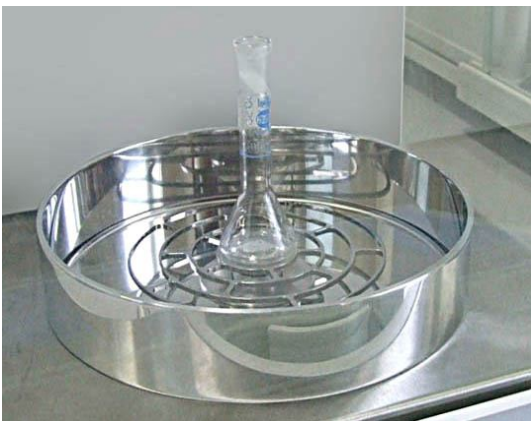
Grid weighing pan, external shield of the microbalance
