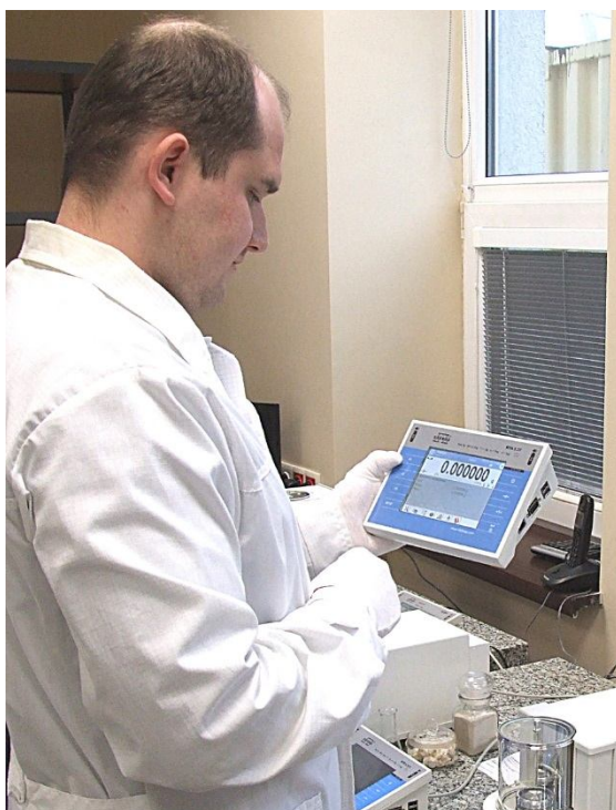
Fig. 76. Balance-terminal wireless connection
