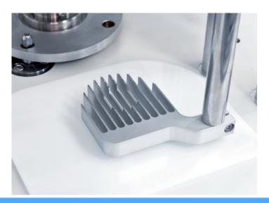
Thanks to a special structure of the insert, the comparator offers a wide measuring range (from 1 q to 1 kg) and is adapted to comparing silica hemispheres.
