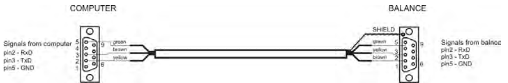
Balance – computer cable (RS232)
