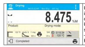
Upon drying process completion, summary of the test is displayed, final moisture content result is held, drying chamber's lid gets opened automatically. Upon process stop, printout footer is sent to a selected interface (accordingly to set printout options – parameter group DRYING PROCESS REPORT/FOOTER).
