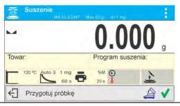
Indication equals ZERO, drying chamber's lid gets opened automatically, subsequent prompt is displayed and the pictogram on drying chamber status changes.
