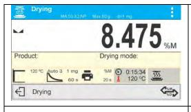
In course of a drying process current weight results and information on the process is displayed (test duration, drying chamber temperature, etc.). In course of a drying process (accordingly to set printout options – parameter group DRYING PROCESS REPORT/MEASUREMENT) measurements are sent to a selected communication port in a preset time intervals (INTERVAL).
