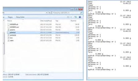
The data can be printed using any computer-connected printer. It is possible to overwrite the file with new data therefore you can continue recording measurement data using the file once created.
