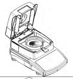
Load the weighing pan with the sample. Sample mass shall be selected on the basis of prior experience and tested material characteristics.
