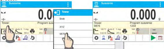
5.In addition, the BIAS function can be used when selecting products. This is a function that enables the drying result to be automatically corrected and the corrected value to be displayed in the information field during drying.
