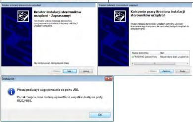
2. Having completed driver installation, connect the moisture analyzer to a computer, use maximum 1.8-meter long USB A/B cable (if the moisture analyzer is already connected, disconnect it, next reconnect it using USB cable).
