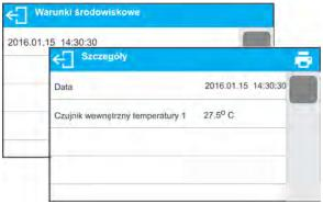
Caution: The software saves ambient conditions record in a so called loop, i.e. when the measurement 10 001 is saved, the measurement 1 gets automatically deleted from the moisture analyzer memory.
