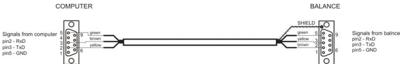
P0108 Kabel Waage – Computer (RS232)
