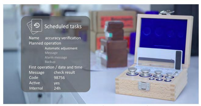
Figure 8. Mass standard set adopted for periodical inspection of balance
