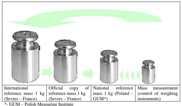
Fig. 2 Visualization of measuring retraceability as in case of reference mass
