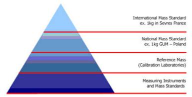
Fig. 3 Schema of measuring retraceability
