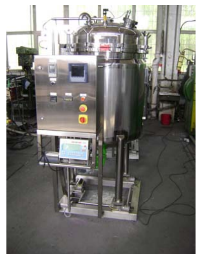
Fig 3. Dosing of pharmaceutical substances using PUE C41H
