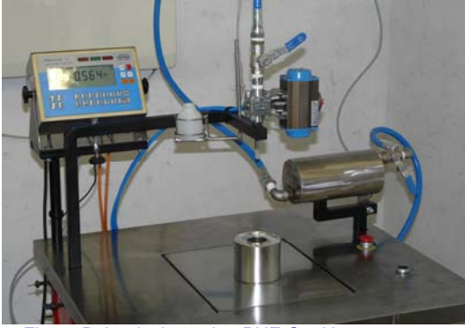
Fig. 4. Paint dosing using PUE C41H
