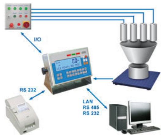
Fig.1: A system diagram – dosing with recipes on the basis of the PUE C41H terminal
