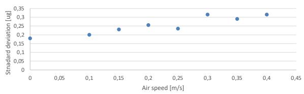
As you can see, the repeatability of the comparator increases almost linearly with the increase in air movement.
