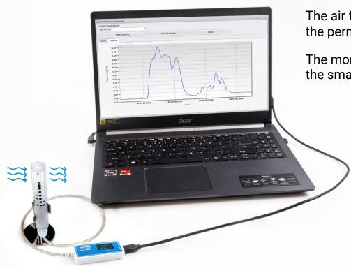
The air flow indicator informs the user about the permissible air flow level in m/s.
