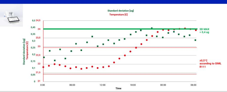
The comparator tested by using an internal adjustment standard during weekend without the presence of people and with a programmed temperature change, showed a slight increase in repeatability by the dynamic temperature change. Due to its structure and lower resolution (50 million units), the comparator is quite resistant to sudden temperature changes.
