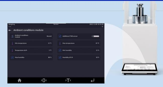
The program calculates the final calibration result together with estimation of the measurement uncertainty consistent with the OIML R-111-1 recommendation. RMCS contains a database of limit errors permissible for individual masses and classes of standards in accordance with OIML R-111. It also allows to define own value of a permissible error for the nontypical standards.
