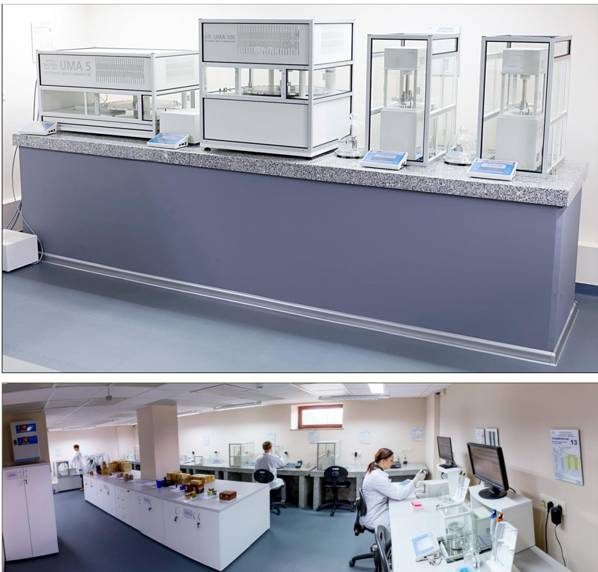
Figure 6. Testing stand for mass comparators/ general view of the laboratory
