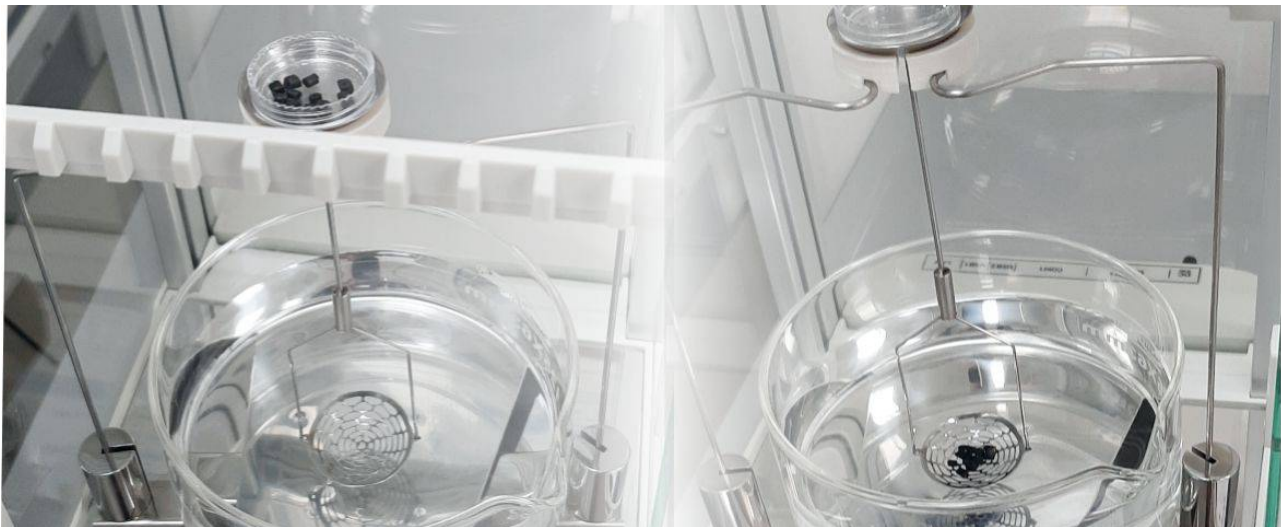
Figure 4. PA 6 GF 15 granule testing in distilled water Measuring the sample mass in the air and liquid on the lower weighing pan
