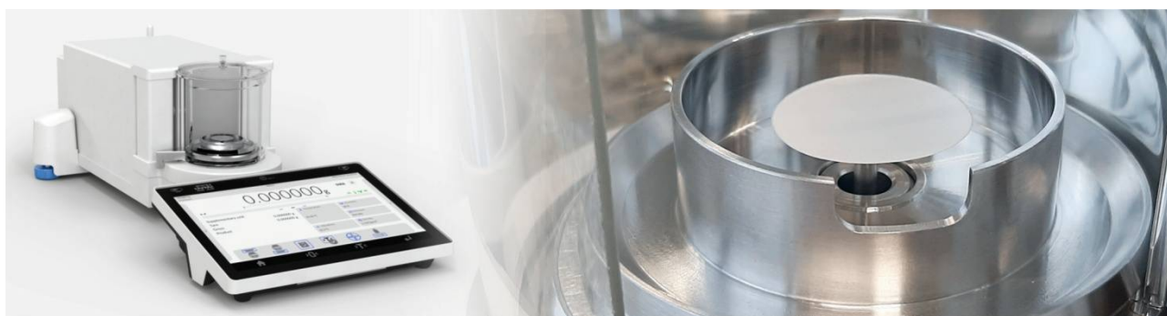
Figure 33. MYA 5.5Y Microbalance , Max 5g, Readability d=1\mu\text{g} , Precision St. Dev.= 0.5\mu\text{g} , Automatic Internal Adjustment, OIML Cert., weighing Chamber optimized for \phi 25 mm filters
