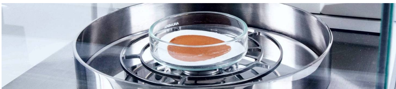
Figure 23. Manual Weighing of a Filter Paper for Suspended Solids Determination in a Wastewater Treatment Plant Using an XA 82/220.5Y Analytical Balance
