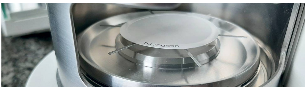
Figure 16. Manual Filter Mass Measurement Using the MYA 5.5Y Microbalance
