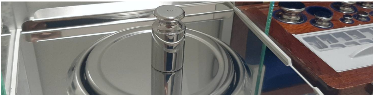
Figure 14. Factory Adjustment Using Certified Mass Standards
