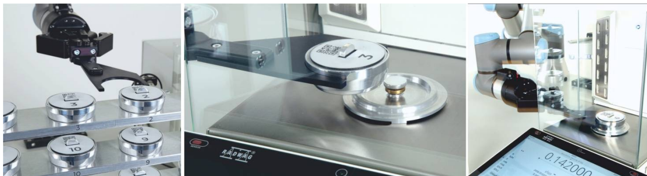
Figure 51. Stages of Cobot Operation: Filter Cassette Pickup and Mass Measurement.
