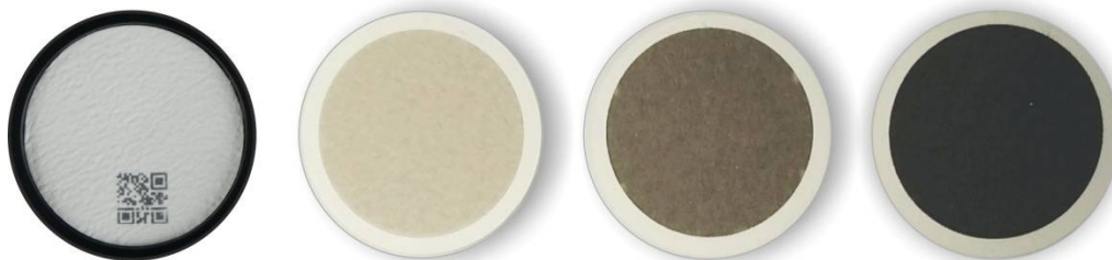
Figure 46. Filter Before Exposure with a QR Code, Filter Placed in an Antistatic Cassette, and Filters After Exposure
