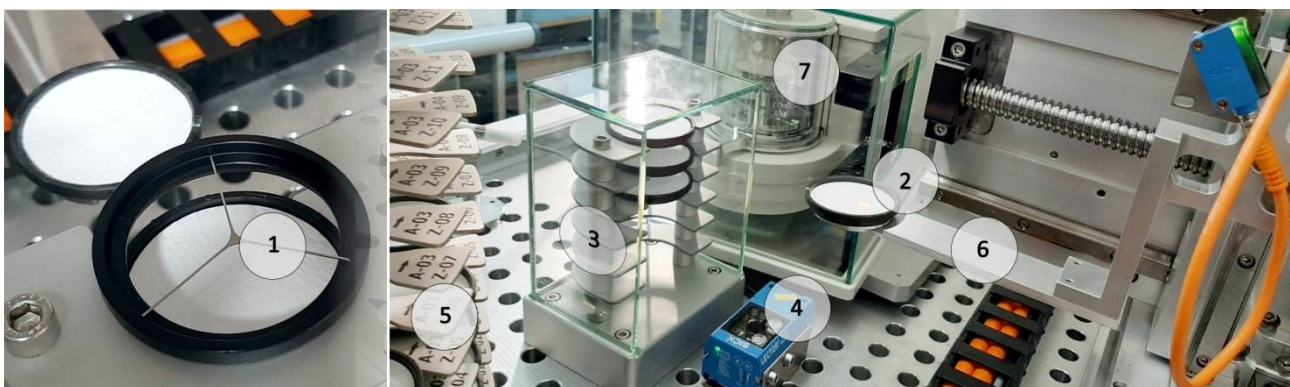
Figure 2. Automation of Mass Measurement – RB 2.5Y Robotic Weighing System
