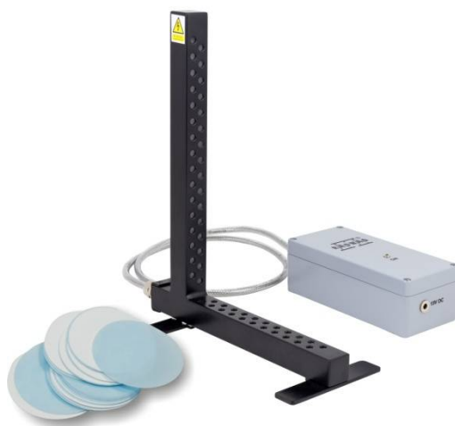
Figure 53. External DJ-05 Deionizer, 12 VDC power supply, stainless steel ion emitter, recommended sample-to-deionizer distance during deionization: 5–50 mm.
