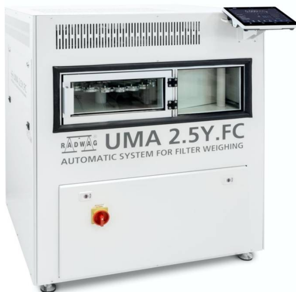
Figure 39. UMA FC Automated System for Monitoring Filter Mass Changes, Filter Conditioning with Controlled Temperature and Humidity, Maximum Capacity 2g, Readability d=1\mu\text{g} or 0.1\mu\text{g} , Capacity up to 24 Filters, Compliant with EN 12341:2024
