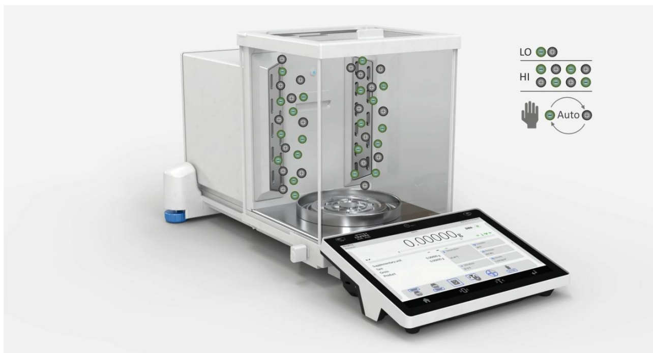
Figure 55. XA 210.5Y.A Analytical Balance with Integrated Ionizer, Max 210 g, readability d=0,01mg, automatic internal adjustment, OIML certified. Compliant with EN 12341:2024
