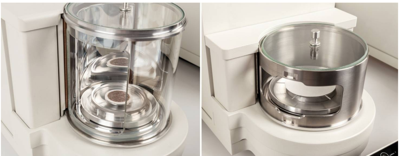
Figure 26. MYA 5.5Y and MYA 5.5Y.FA Microbalances with a readability of 0.001mg
