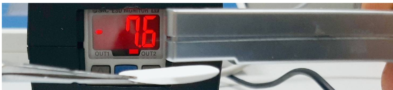
Figure 52. Measurement of Electrostatic Charges on a Filter Using an SMC IZD10-510 Meter
