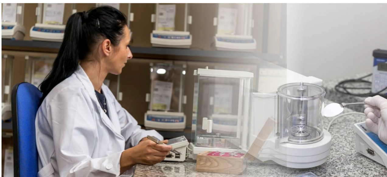
Figure 27. Verification of Balance Indication Accuracy Using Certified Mass Standards in the Radwag Quality Control Department and Filter Weighing as a Qualitative Assessment of Balance Performance for Laboratory Applications
