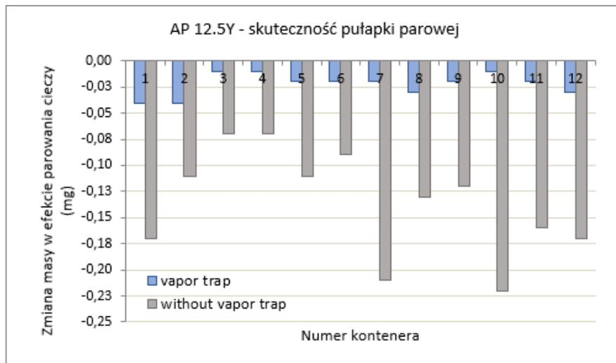
Photo 24. Liquid evaporation from the weighing vessel in the AP 12.5Y system
