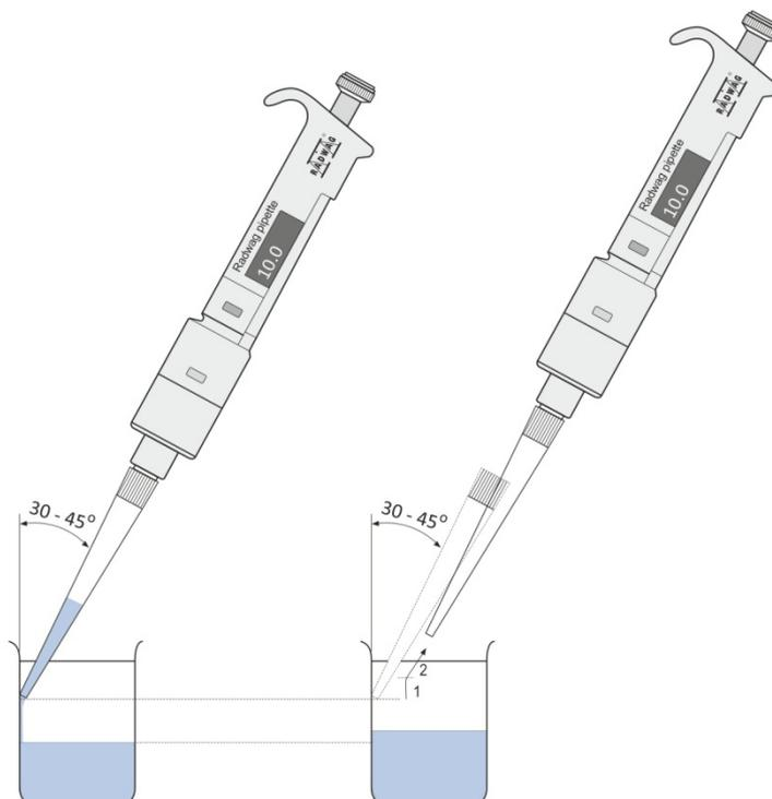
Photo 18. Method of expelling liquid from pipette
