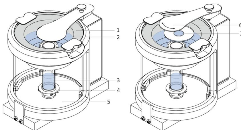
Photo 7. Automatic chamber for pipetting with the use of XA balances
