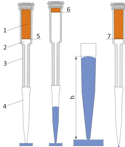
Photo 29. Piston pipette - liquid collection stages
