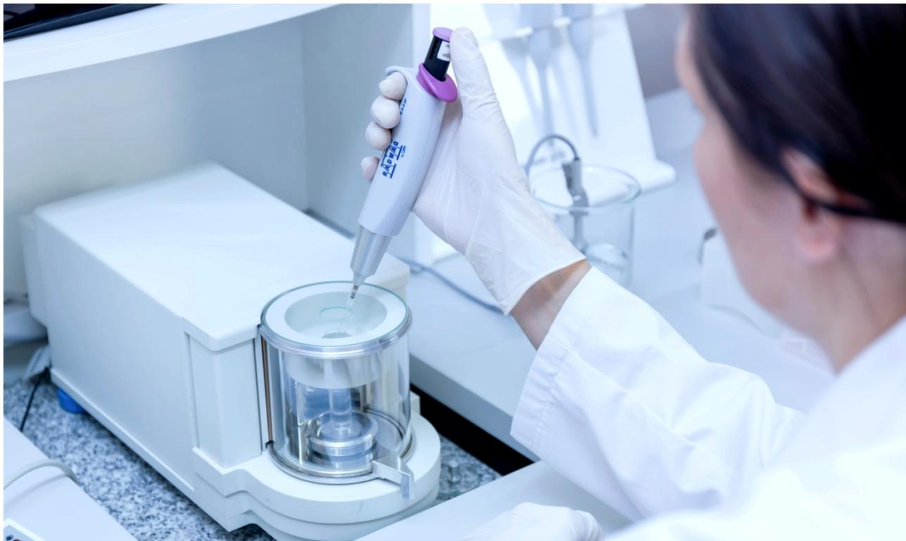
Photo 9. Inspecting piston pipette volume with the use of MYA microbalances
