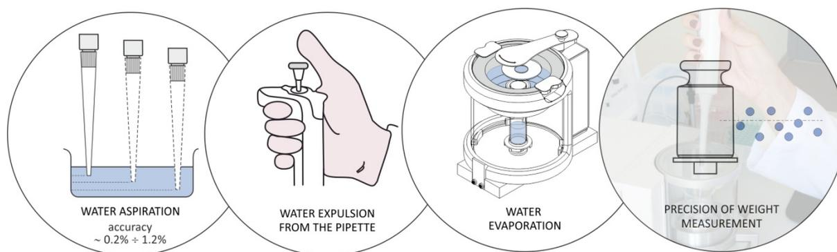
Photo 14. Sources of errors while pipetting
