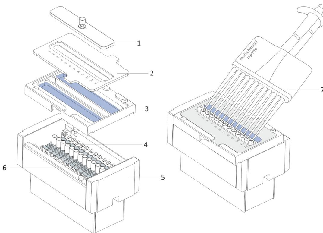
Photo 13. Components and design of the AP 12.5Y automatic unit
