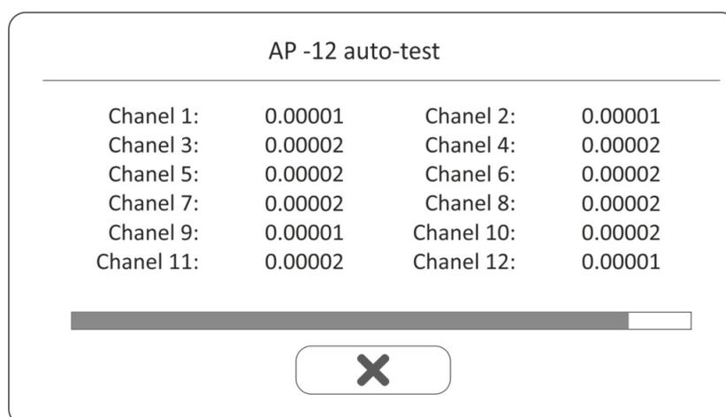
Photo 19. Results from the automatic control procedure – standard deviation from 10 measurements
