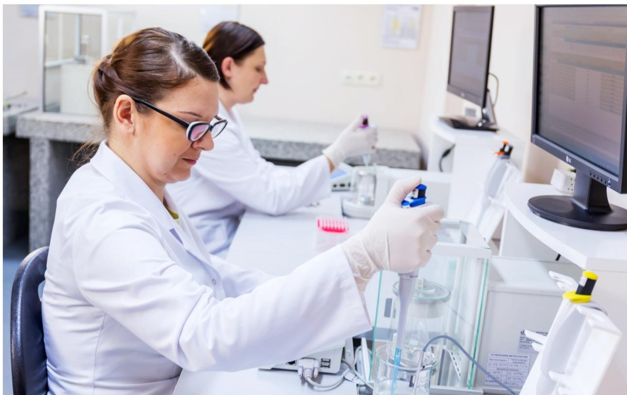
Photo 3. Piston pipette inspection – measuring position for XA balances and MYA microbalances
