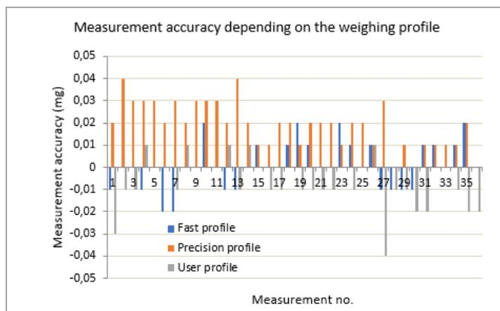
Photo 21. Precision of measuring container mass in the automatic cycle
