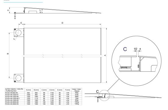
Ramps made of stainless steel
