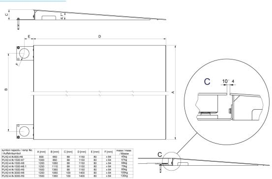
Ramps made of stainless steel
