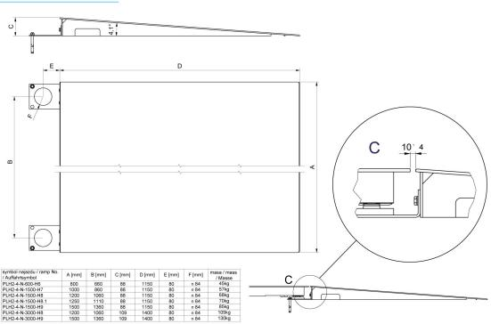
Ramps made of stainless steel
