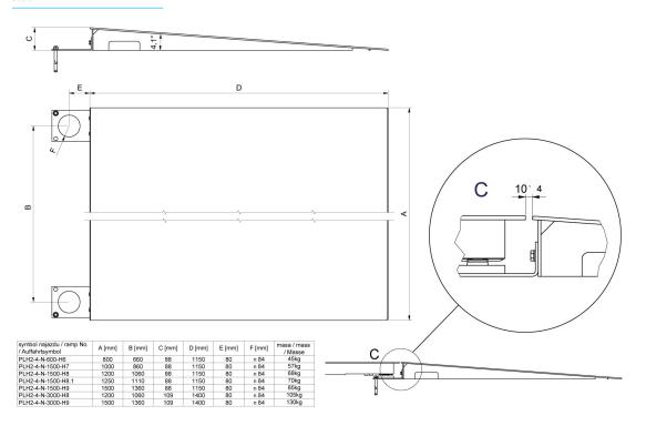
Ramps made of stainless steel
