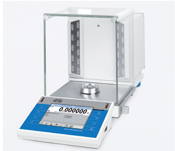
XA 4Y.M.A.I balance with an integrated antistatic ionizer and weighing chamber featuring automatic door
